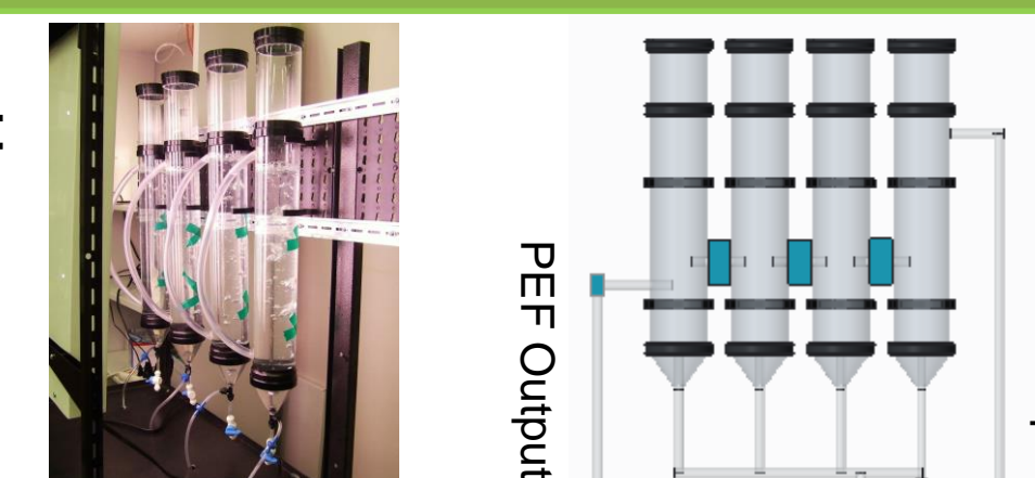
Figure 3. (Right) Constructed airlift, (Left) airlift CAD.
